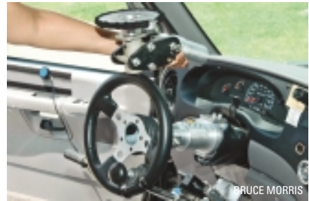
Left: The Digi-Pad system controls vehicle operations; right: VA offers six different steering wheel orientations based on the patient’s specific needs.
